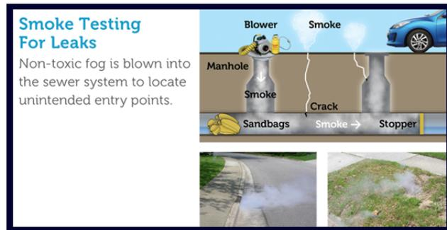
If the sewer line is in good condition and there are no problems to be fixed, the only places smoke should exit are sewer vent pipes. Any other places that smoke escapes indicate a problem with the sewer system in that area.
