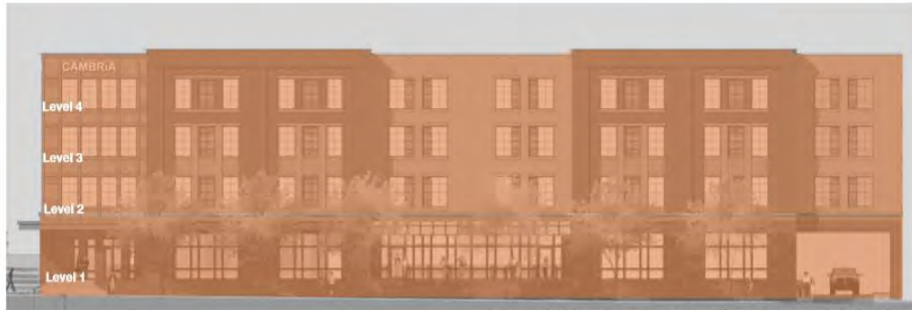
The red area denotes the building's pedestrian storefront. The areas of glazing are calculated from this portion.
